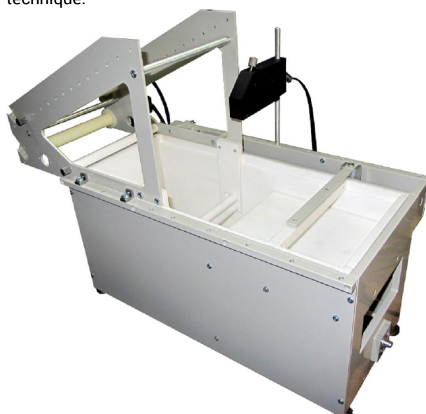
Configuration of the trough for horizontal precipitation includes horizontal barrier, surface tension sensor and specialized rig – two Z-shaped PTFE bars with adjusting screw on one end. Draining hose(s) are employed in the technique.
