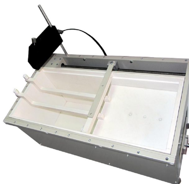
Configuration of the trough for horizontal precipitation includes horizontal barrier, surface tension sensor and specialized rig – two Z-shaped PTFE bars with adjusting screw on one end. Draining hose(s) are employed in the technique.
