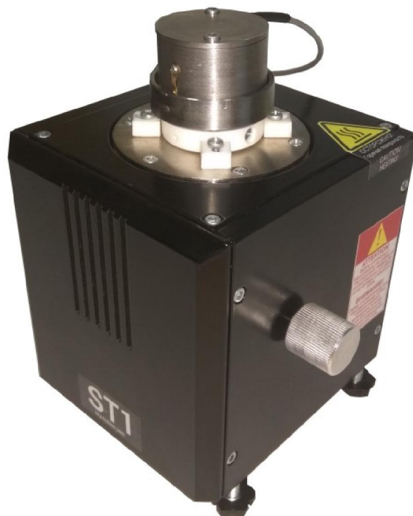
Fig. 1.4. The measuring unit. Holder of upper electrode installed in regular position (case of the integrated preamplifier is above the unit upper cover). Knob of hoist gear mechanism to lift/sink lower electrode is on the unit right wall
