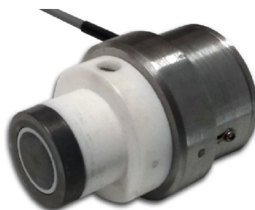
Fig. 1.6. Upper electrode holder with integrated preamplifier of pA-range signal
