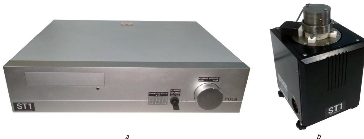
Рис. 1.1. General view of instrument for measurement of thermostimulated current ST1: a – control electronic unit; b – measuring unit
