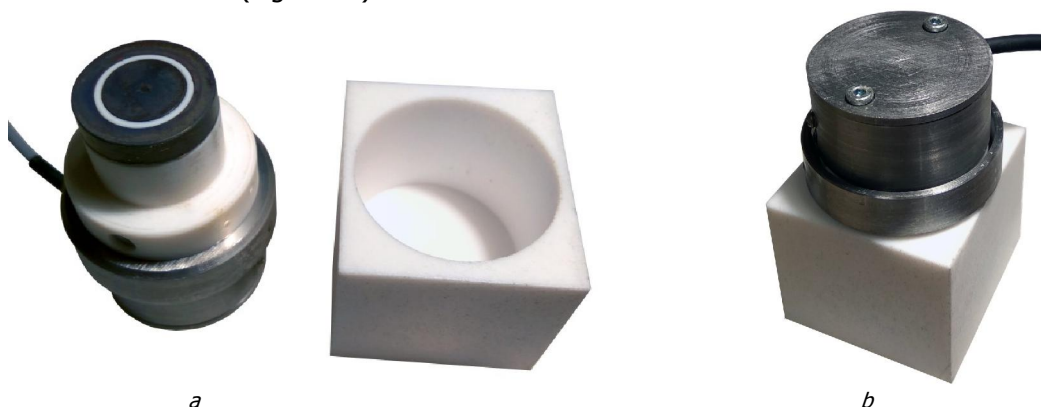
Fig. 1.7. Safe placement of the upper electrode holder: a – on the preamplifier case top with the electrode upward (PTFE shell from the shipment set shown on the right); b – inside PTFE shell from the shipment set
