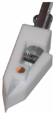
Fig. 1.5 – A PTFE holder for substrate clamping.
