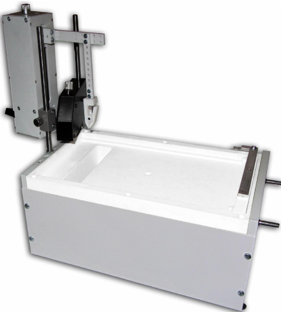
Fig. 1.6 – LB trough filled with liquid and equipped with surface pressure sensor and dipper unit bearing substrate ready for operation. Barrier is in rightmost (initial) position.
