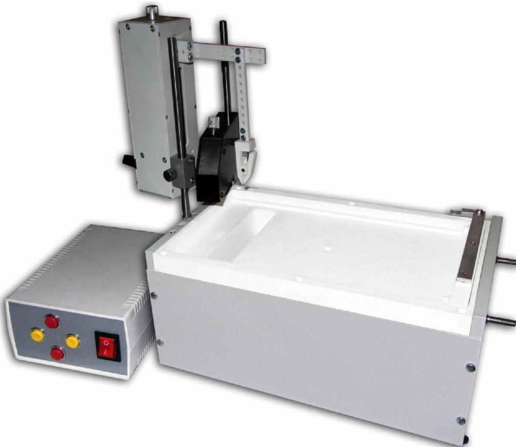
Fig. 1.1 – General view of the Langmuir–Blodgett trough LT-111. Right – control electronic unit, left – LB trough.
