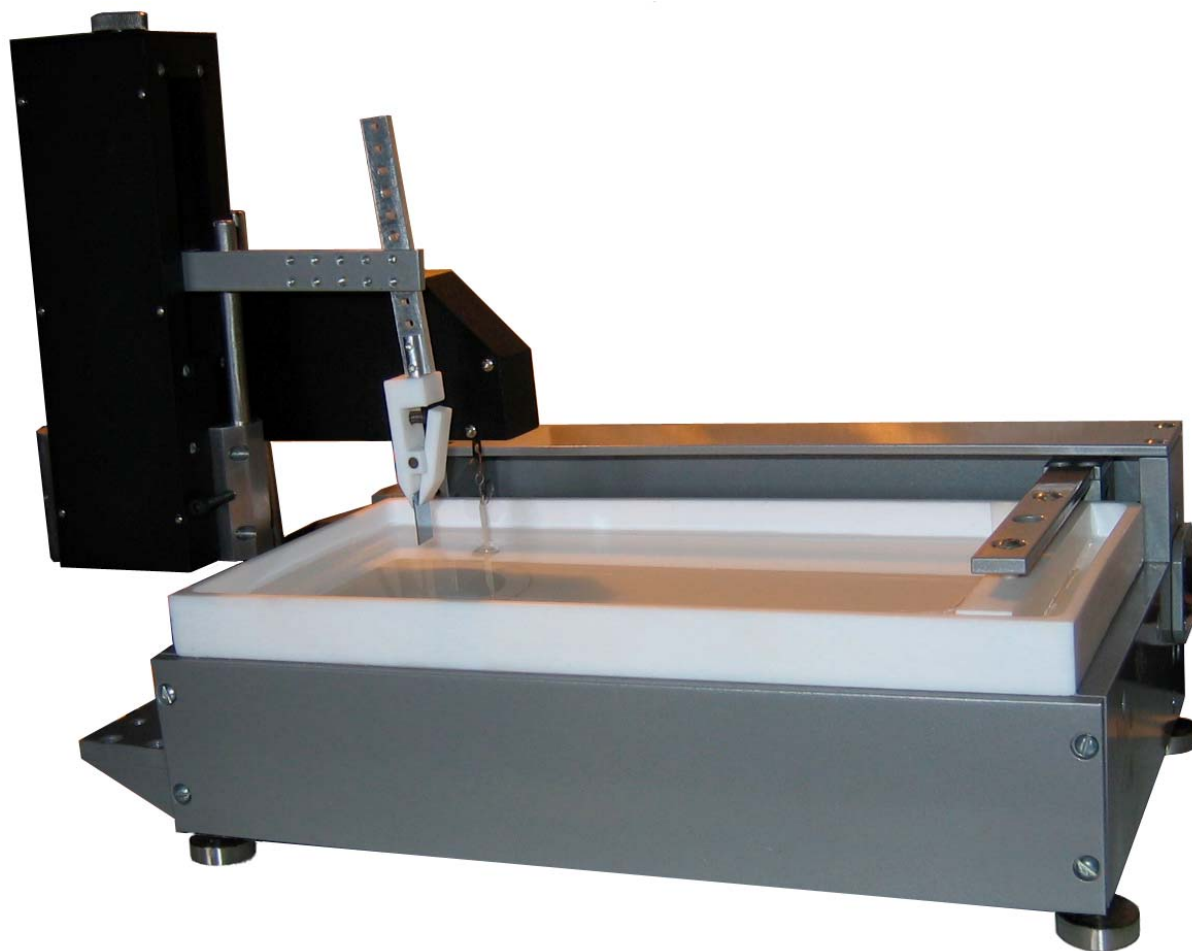
Fig. 1.6 – LB trough filled with liquid and equipped with surface pressure sensor and dipper unit bearing substrate ready for operation. Barrier is in rightmost (initial) position.
