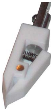
Fig. 1.5 – A PTFE holder for substrate clamping.
