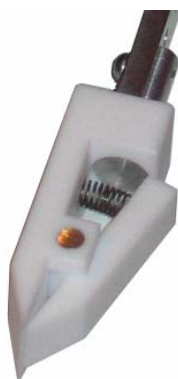
Fig. 1.5 – A PTFE holder for substrate clamping.
