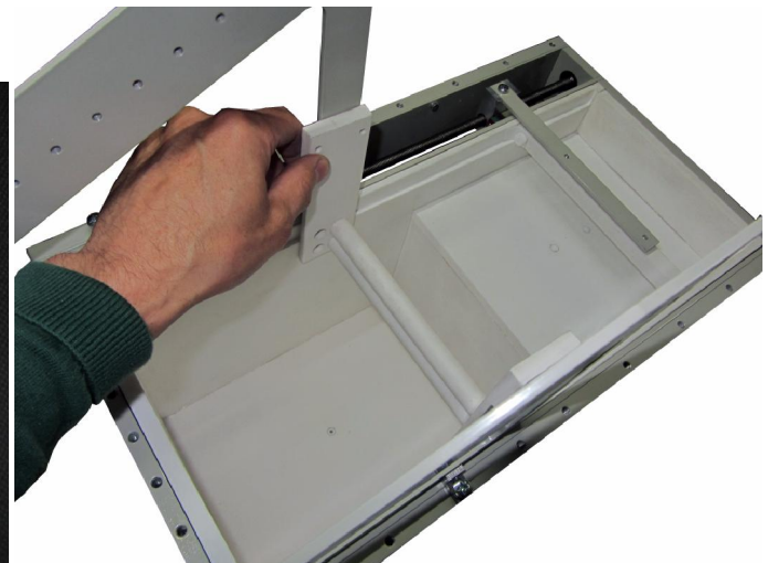
3.4. Insert one or two PTFE guides to the PTFE holders and insert all them into dipping well. The guide(s) will organize motion of the submerged portion of the tape substrate
