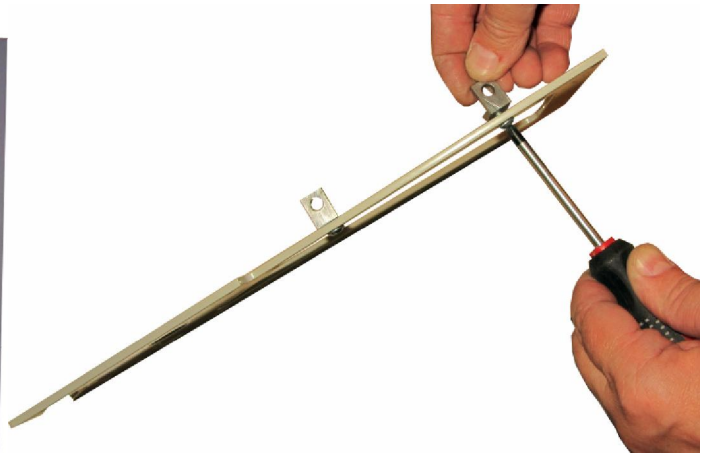
3.3. Mount rear and front frames of the tape winding set on the trough using M6x12 screws.
