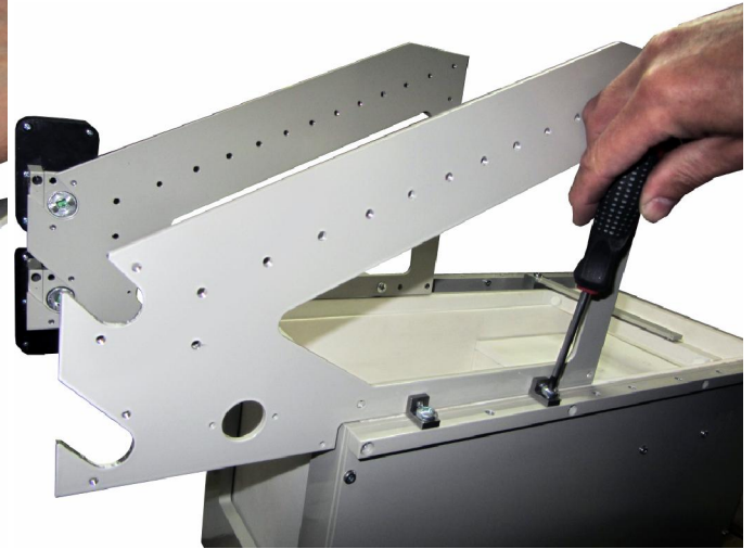
3.4. Insert one or two PTFE guides to the PTFE holders and insert all them into dipping well. The guide(s) will organize motion of the submerged portion of the tape substrate
