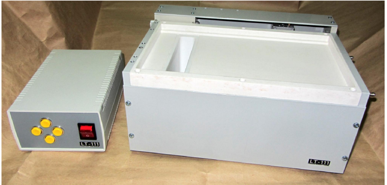
After unpacking the box with LT-111: Control electronic unit (left) and LB trough (right)
