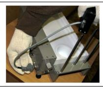
4. Adjust vertical position of the surface pressure sensor unit and fix it with a clamping screw on the mounting rod.
