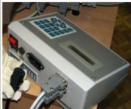
11. Place the assembled device onto its working location. Connect the control unit to host PC with the USB cable. Install the LB trough control program onto the PC (use a CD placed before rear cover of the manual). The device is ready for further operation.
