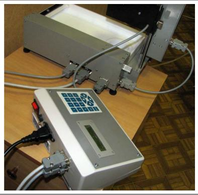
Note, careful washing of the PTFE trough and barrier is regular operation and should be thoroughly done before the first filling of the trough with liquid.
