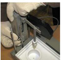
7. Using the cable from the delivery set, connect dipper unit to the connector on side wall of the trough (under the barrier drive knob).
