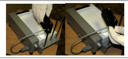
5. Install the dipper arm in working position: screw the horizontal arm to the block on the unit and then fix vertical bar with substrate clamping holder.
