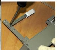
6. Mount the dipper unit on middle stand, adjust its vertical position and fix with the clamping screw.
